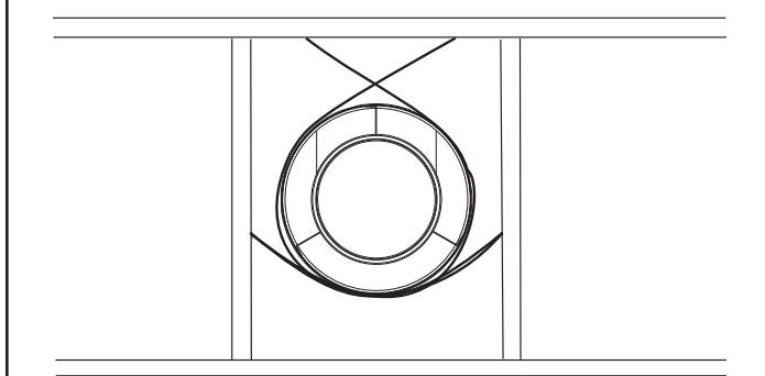
Figure 3.7 - Securing Horizontal Pipe Sections
