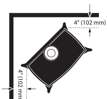
Figure 2.4 - Corner installation, minimum corner clearances.
