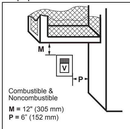
**\*NOTE:** Termination in an alcove space (spaces open only on one side and with an overhang) is permitted with the dimensions specified for vinyl or non-vinyl siding and soffits.
