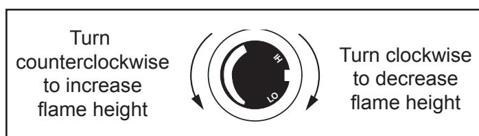
Figure 4.3 - Flame adjustment knob for SIT valve.
