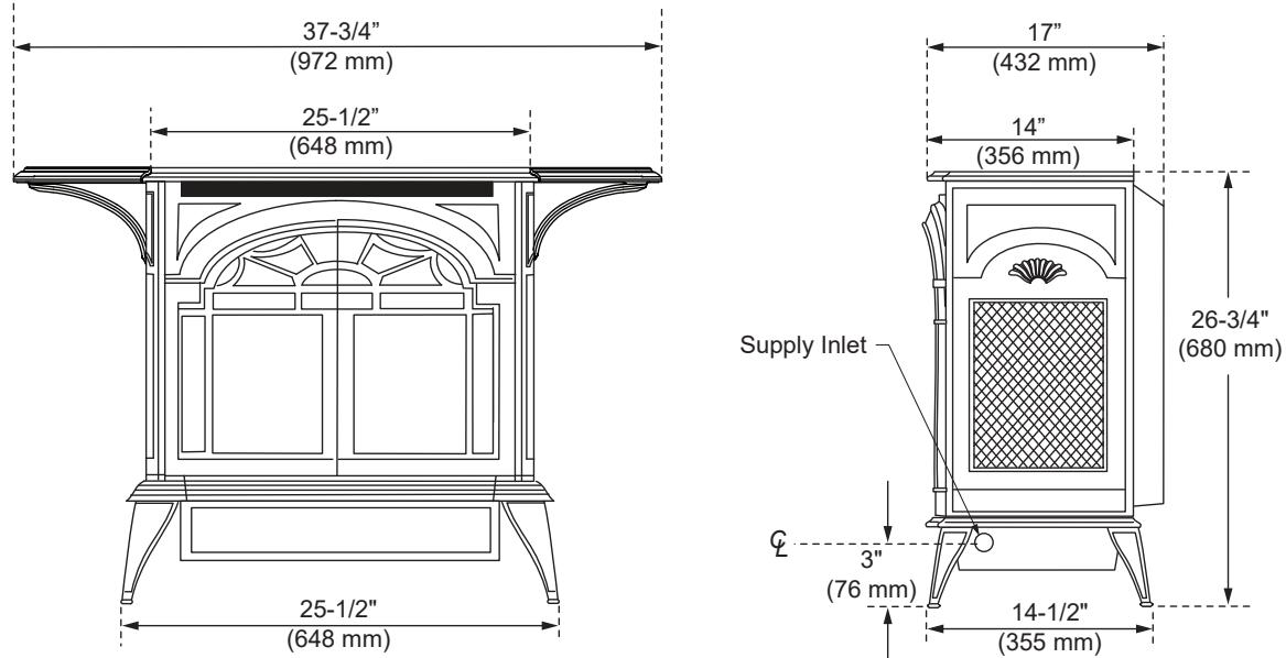
Figure 2.1 - Stardance dimensions. Weight: Fully assembled; 202 lbs.
