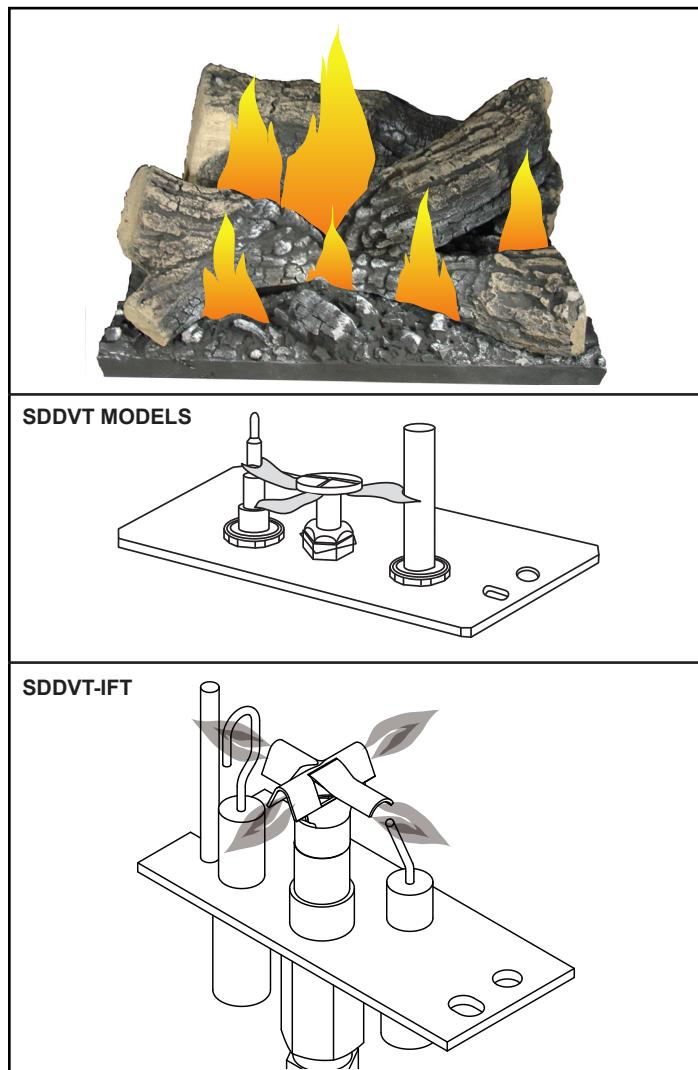
Figure 4.2 - Correct pilot and burner flame appearance.
