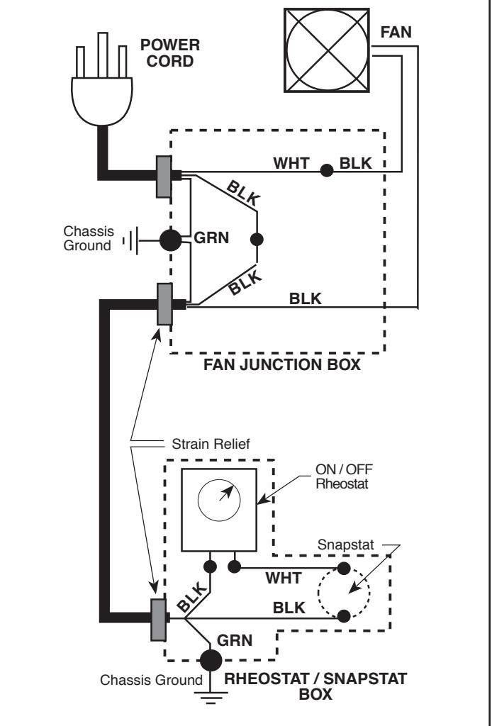
Figure 6.2 - Fan circuit.
