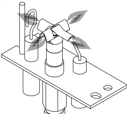
Figure 4.6 - Correct pilot and burner flame appearance.
