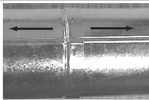
Figure 3.9 - Align and Disassemble Vent Sections
