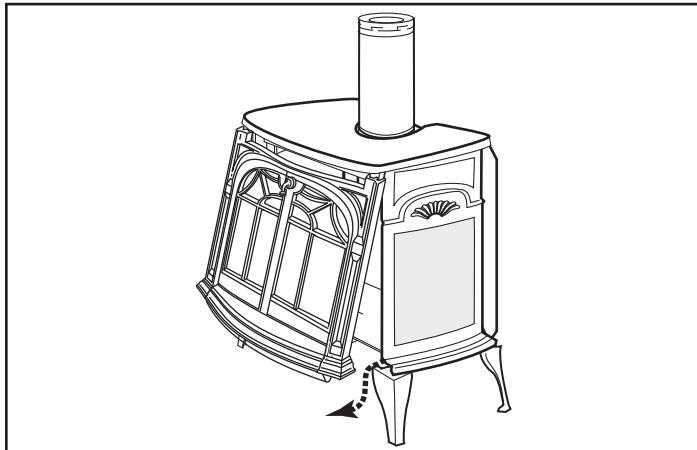
Figure 3.24 - Remove the safety barrier and stove front.
