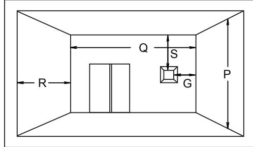
$$Q_{\text{MIN}} = 3 \text{ feet} \\ (0.9 \text{m}) \quad R_{\text{MAX}} = 2 \times Q_{\text{ACTUAL}} \quad R_{\text{MAX}} \leq 15 \text{ feet} \\ (4.6 \text{m})$$
