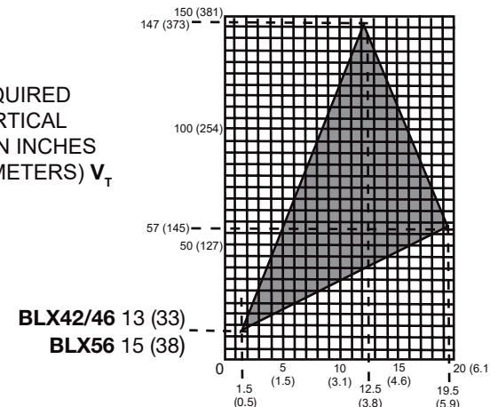
HORIZONTAL VENT RUN PLUS OFFSET IN FEET (METERS)  $H_T$
