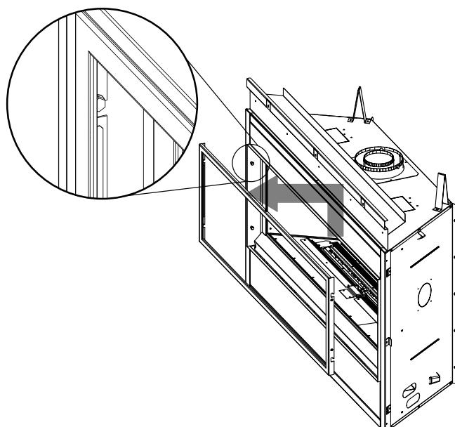
Before the glass door can be removed, the safety barrier must be removed. Lift the safety barrier off the four shoulder screws and remove from the appliance.
