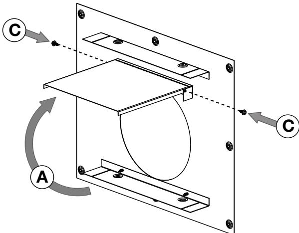
When using flex venting, use firestop assembly:
