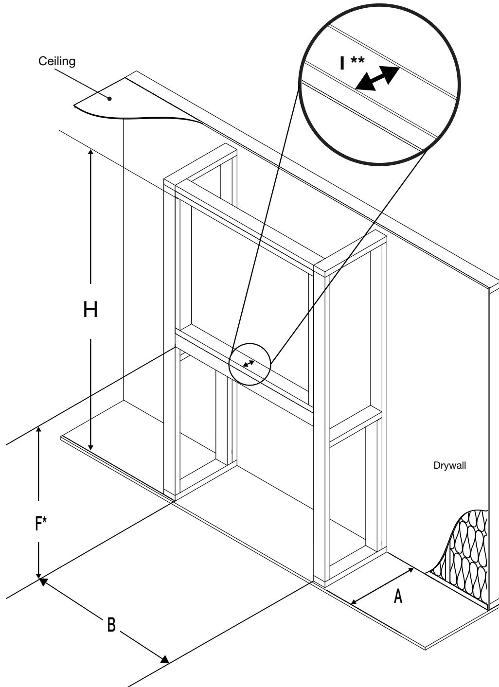
\* Allow for finished floor and hearth thickness when setting these dimensions.
