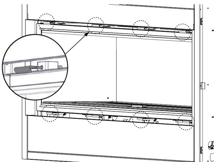
Leave a hand on the glass door during entire door removal. The glass door is secured to the firebox with four (BLX42), six (BLX46), or eight (BLX56) spring latches. Pull the handles of the latches forward, then lift/lower the latches out from the door frame to release the door. Next, lift the door up until the bottom edge clears the bottom shoulder screws of the appliance. Carefully grip the top and bottom of the door lifting it off the appliance.
