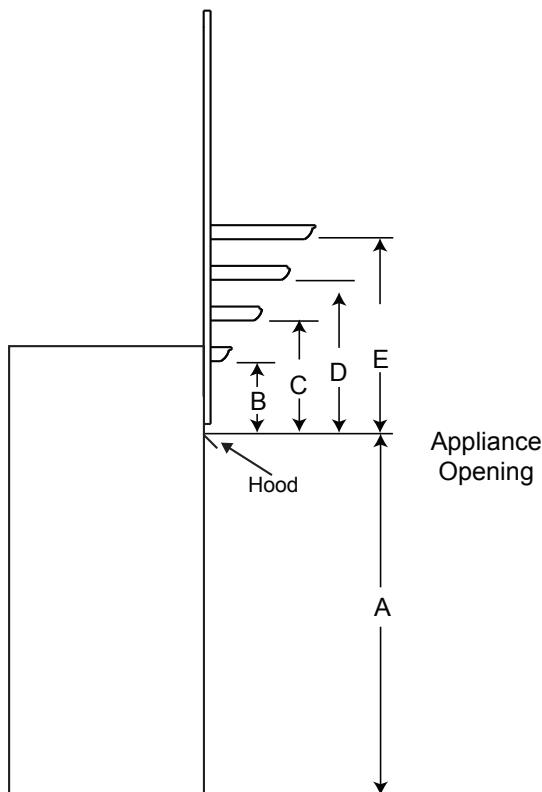
**ONLY if the Universal Heat Management System is installed, mantel clearances can be reduced.**
