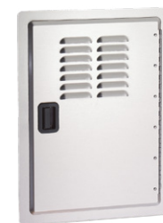
20-14-SDV 20" x 14" Access Door w/ Louvers • Cut-out: 20½" h x 14½" w
