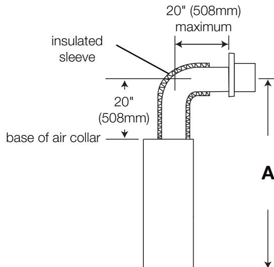
Use the periscope kit to locate the air termination above grade. The periscope must be installed so that when final grading is completed, the bottom air slot is located a minimum 12" (305mm) above grade. The maximum allowable vent length is 10' (3m) for a fireplace and 8' (2m) for a stove.
