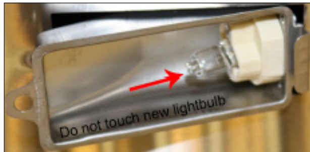
4. Replace light bulb 5. Reverse process to replace into housing
